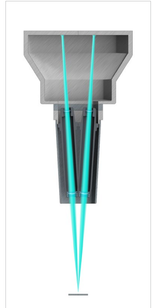
Beam path of a Greenough type stereo microscope
